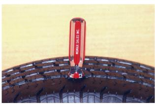
4. ...until handle is flush with the tire. (CHEMI CURE can also be used for rim leaks.)
