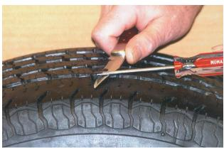
6. Withdraw tool slowly just until the end of the tool clears the tire. Cut repair flush with tire surface.
