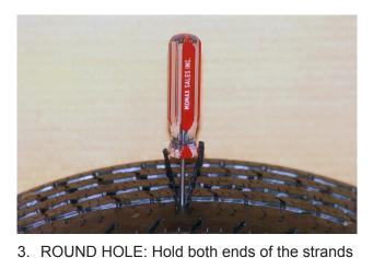
against one side of the tool. Insert tool slowly all the way into the puncture...
