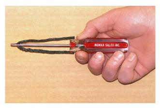
1. TO THREAD TOOL: Put a strand into eye of tool and with thumb and index finger slide tool eye to the center of the strand.
