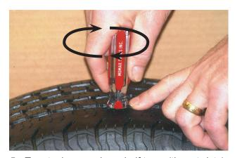
5. Turn tool one and one half turns (three twists).
