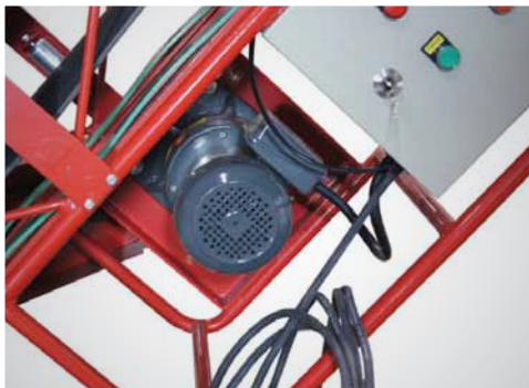
Tire conveyor motor 1,5HP or 2HP (depending on the conveyor model)
