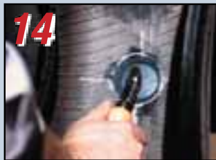
14 After the repair unit is applied, stitch thoroughly from the center outwards.
