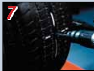
7 Ream the tire injury (from the outside), using a carbide cutter with a low speed buffer.
