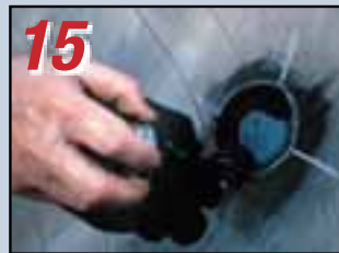
15 Apply REMA TIP TOP Repair Sealant over the repair unit and buffed area.
