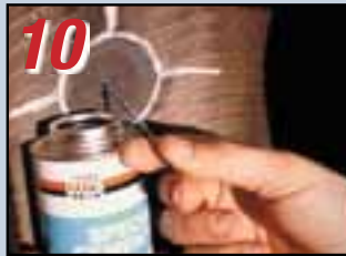
10 Apply REMA TIP TOP Blue Cement into injury channel with a 626 pull-wire.
