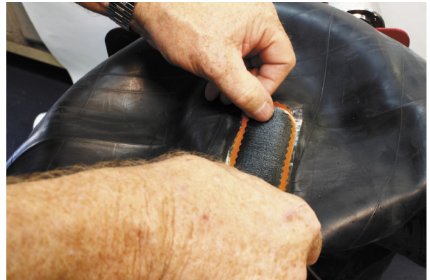
10. Remove the protective foil from the back of the Repair Unit and apply over the injury / cemented area. Avoid touching the Repair Unit.
