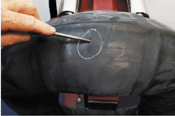
1. Inspect the tube for the extent of the injury.
