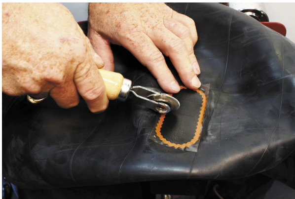
11. Stitch vigorously from the center out to remove any trapped air.
