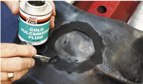
7. Apply a thin application of the proper cement and allow to dry.
