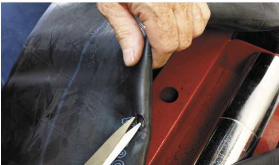
11. Move to the opposite side of the innertube and make a new hole to install the new valve.
