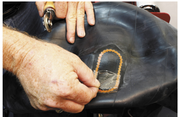
12. Remove the plastic on top of the Repair Unit.
