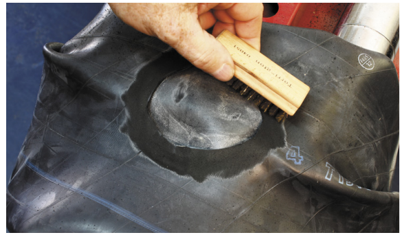
6. Clean the buffed area by using a brass brush.
