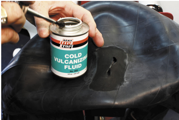
9. Apply a thin application of the proper cement and allow to dry.
