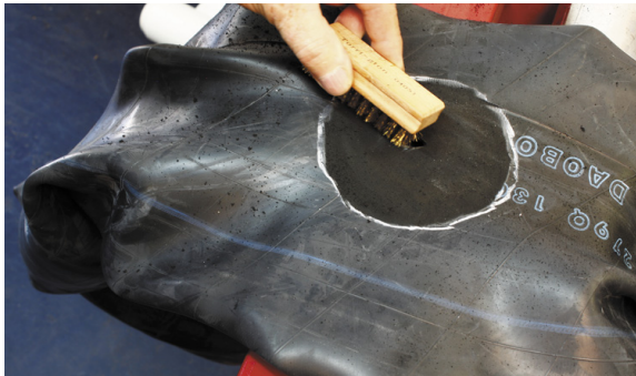
15. Clean the buffed area by using a brass brush.
