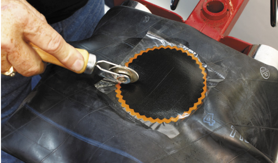
9. Stitch vigorously from the center out to remove trapped air.
