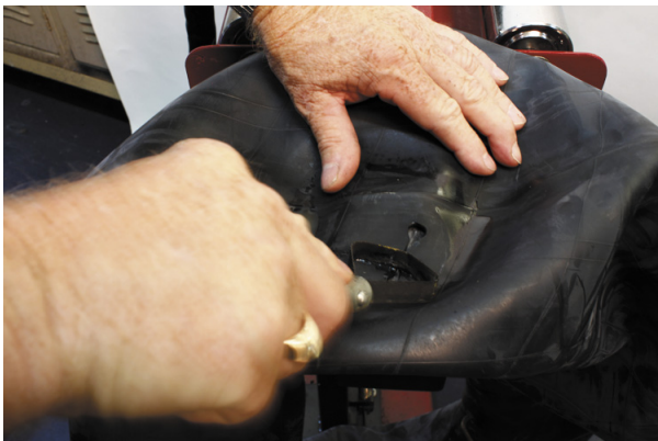
5. Scrape the contamination from the area.
