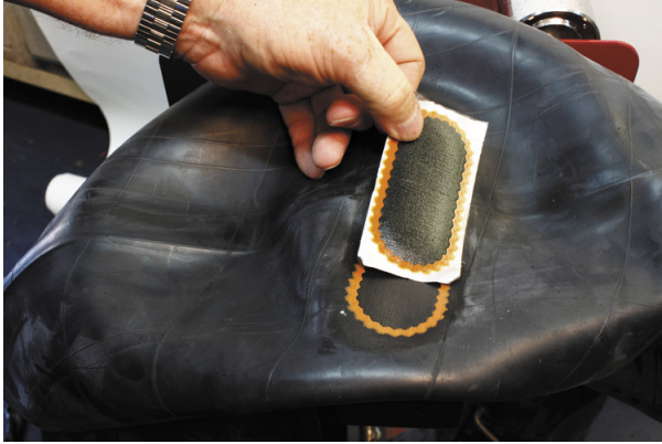
4. Select the appropriate size of tube repair to be used.
