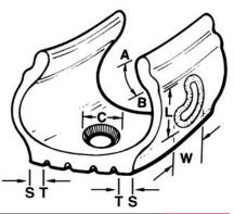
**A-B**-NON-REPAIRABLE AREA **C**-MAXIMUM DIAMETER OF DAMAGED RADIAL CABLES W-WIDTH OF INJURY L-LENGTH OF INJURY S-T - SHOULDER AREA T-T-CROWN AREA
