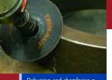
Deburring and chamfering a section of pipe after cutting.
