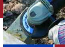
Removing heavy weld spatter while prepping surface for painting.
