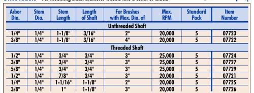
Plastic Adapters - For mounting small diameter wheels onto various arbor sizes.
