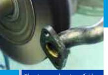
Cleaning an exhaust manifold for a small gasoline engine.
