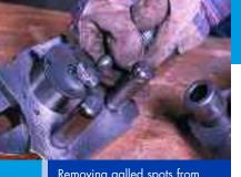
Removing galled spots from a metal forming die.
