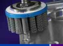
Deburring the edges of an aluminum engine cover.
