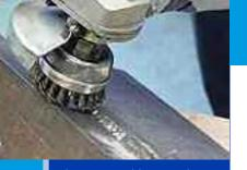
Cleaning a weld joint and removing surrounding spatter with a banded knot cup brush.
