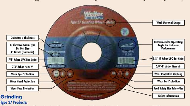
These products range from 4" to 9" diameter and are available in 1/4" thick for grinding and 1/8" thick for light grinding. Type 27 Wheels are offered in aluminum oxide, silicon carbide or zirconium grain with a 5/8"-11 hub option.
