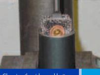
Cleaning the sides and bottom of a deep drawn part using a square brush.
