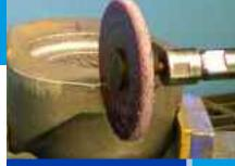
Removing casting flash from ductile-iron housing with an encapsulated brush.
