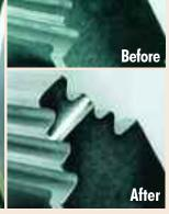
**Problem:** Protecting turbine engine components against high-temperature fatigue is critical to ensure safe, reliable engine operation. Component edges must be burr-free and generally require an edge radius in the range of 0.005" to 0.060".
