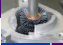
Deburring the internal bores of an air-cooled cylinder head.
