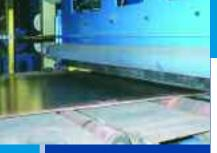
Removing light corrosion and mill scale from coiled steel.
