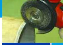
Prepping the bevel end of a stainless pipe for welding.
