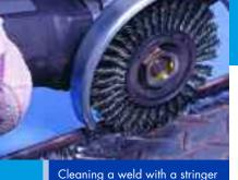
Cleaning a weld with a stringer bead wheel brush.
