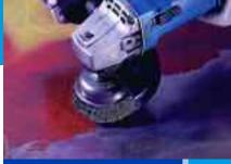
Removing paint from a steel surface with a crimped wire cup brush.
