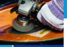
Removing paint from a metal surface with a crimped wire cup brush.
