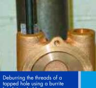
tapped hole using a burrite brush in a holder.
