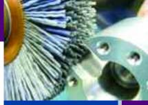
Deburring the edges of a machined aluminum component.
