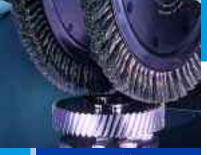
Automotive gear deburring using heavy-duty knot wheel brushes.
