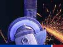
Blending and finishing edges of a flame-cut steel part.
