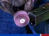
Deburring perforated steel channel after saw-cut.
