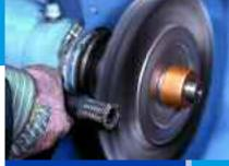
Removing rubber coating from a hydraulic hose.
